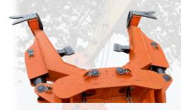
By spreading or closing the arms by hydraulic cylinders, a good break force is created in addition to an enormous clamping force. Because the arms
